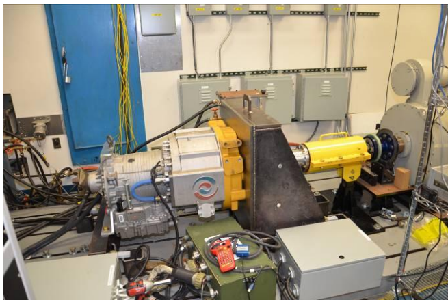
Figure 2 - ISG testing in a SIL at TARDEC
